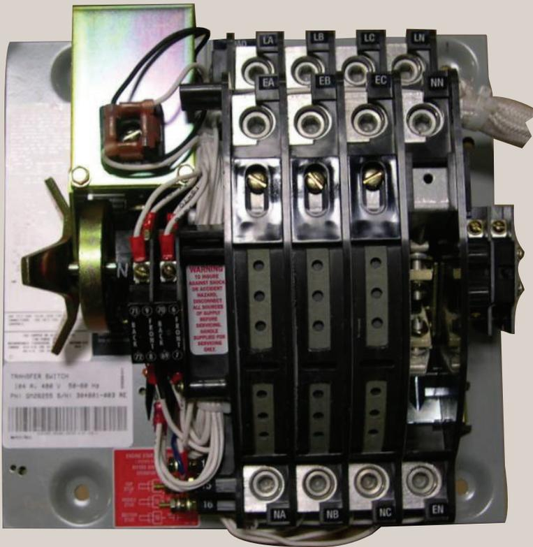
**Summary:** The general rule is when you have a grounded neutral at both the generator and the utility, you must use a transfer switch with enough poles to switch the neutral. If you ground the neutral in both places, you create undesirable multiple paths for ground current to flow.
