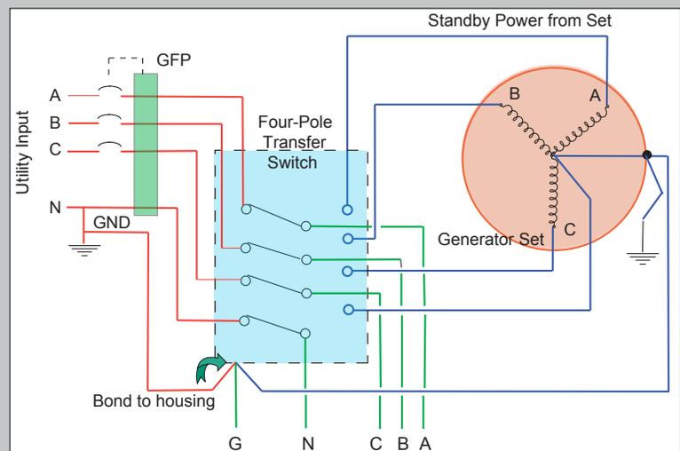
Graphic Two - Detailing System with Switchable Neutral
