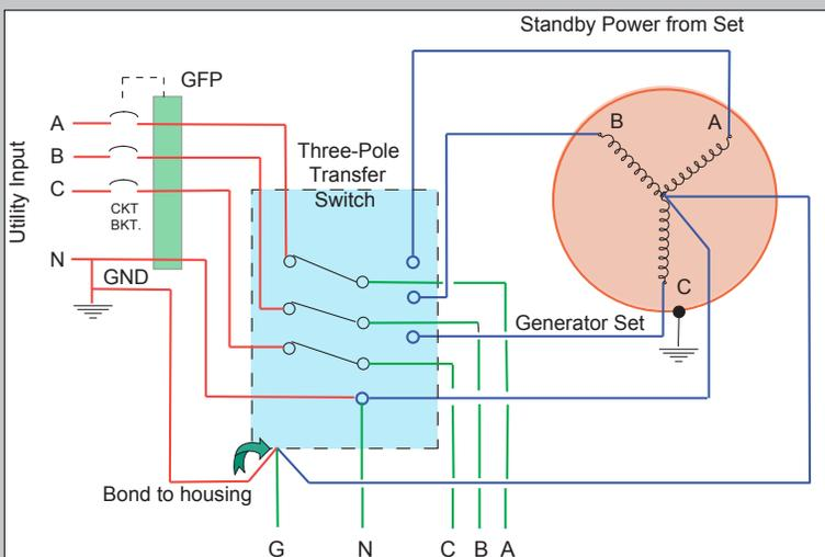
Graphic One - Detailing System with Solid Neutral Connection
